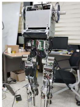
Figure 5.3 Camera mount to combine Gazelle and Kinect V2
