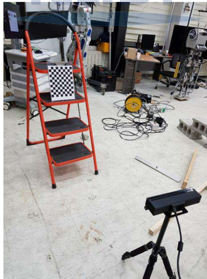
Figure 5.1 Calibrating KINECT V2 with checkerboard.
